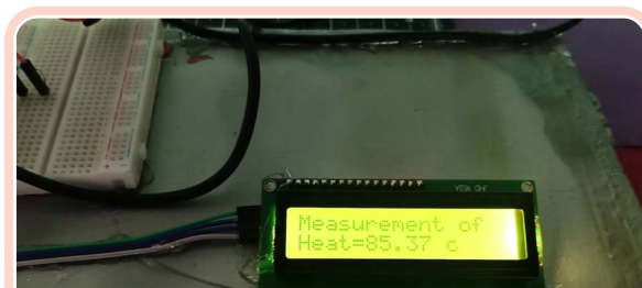
The temperature is still rising indicating the heat generation during the reaction.
