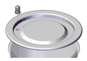
**2.** Take a UV Tube and UV tube holder in 2Qty. Then fixed the UV Tube on Tank Cover using Nuts and Bolts in 4Qty.
