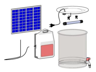
1. Take Stainless Steel Water Tank 20L. Make a 5.30mm hole on Tank Cover for fixing the Wire Glance and also make hole to Tank for Fixing the Water Tap.
