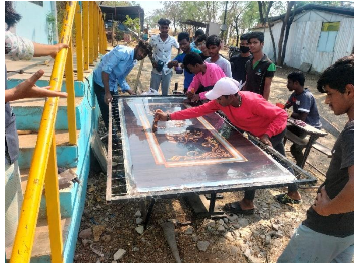
FRP door making
