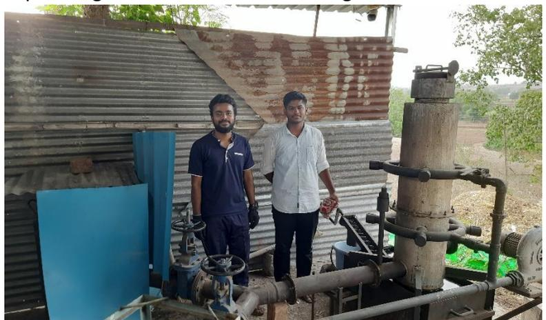
Living lab intern Diwakar kumar tested and experimented with Gasifier sytem using wood chips of different sizes at Pabal
