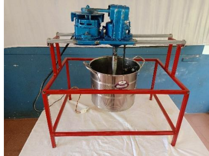
IBT @ Kurdhe (Dist.Ratnagiri) fabricated fruit pulp heating kettle with stirrer arrangement.
