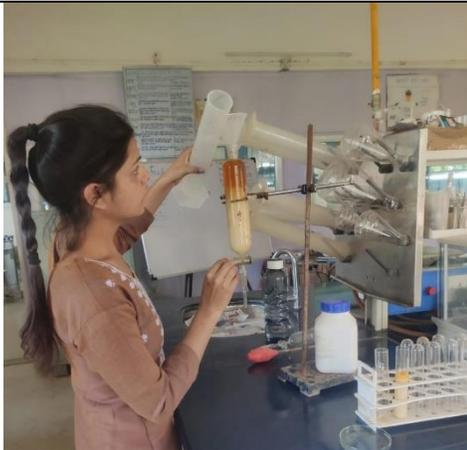
Akshada is using transesterification & fractional distillation process. During 1<sup>st</sup> trial we received 140 ml raw bio-fuel (without fractional distillation) from 200 ml BSF bio-extract. (VATF)
