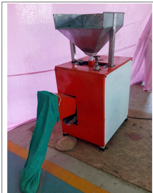
Rice De-husking machine developed for brown rice production.
