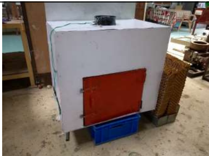
Fabrication of Evaporative cooler under trial
