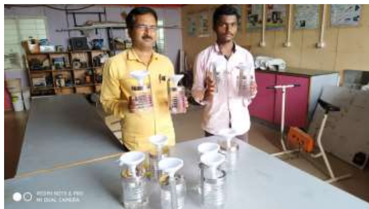
Rain gauges made at ashram
