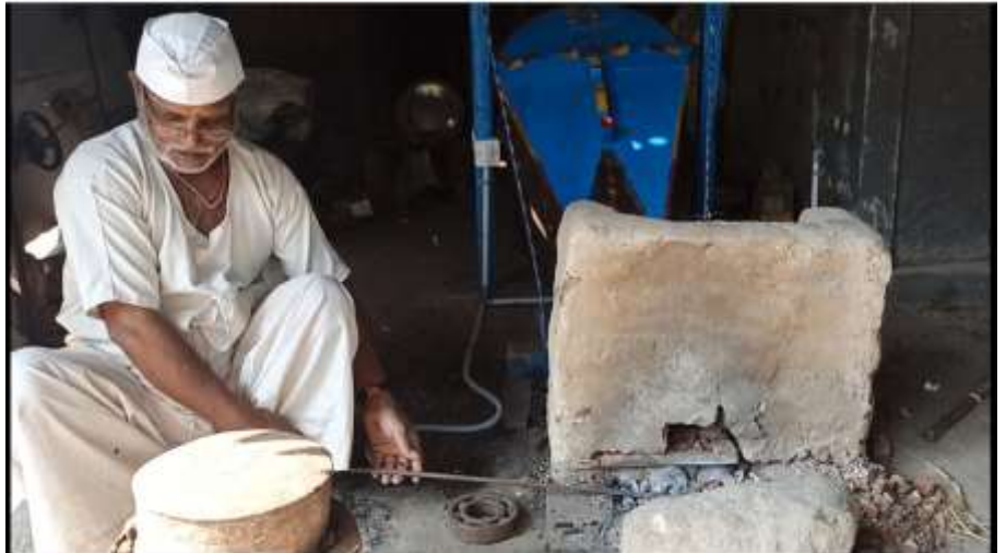
Blacksmithy blower powered by Solar Energy
