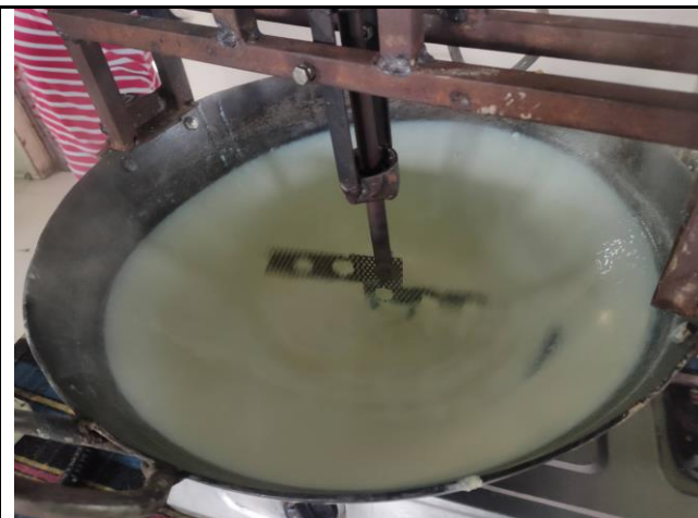
Sanket is working designing khowa kettle' for making khowa and basundi on Solar Concentrator.
