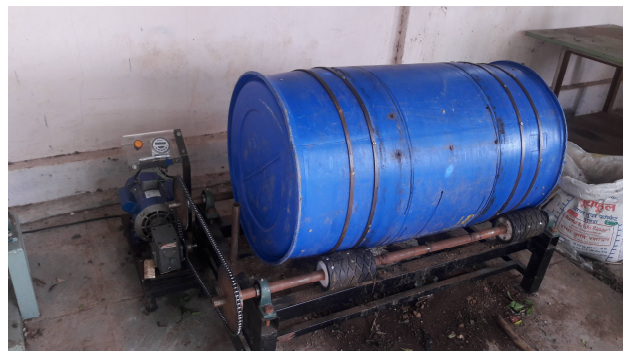
Bio-composter unit : Under testing with 70kg waste for last 4 weeks.
