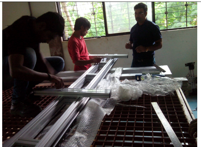
Installation of plasma cutting machine
