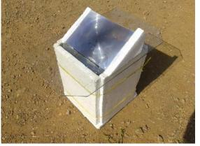
Failed Experiment : Making solar cooker using Fresnel lense.
