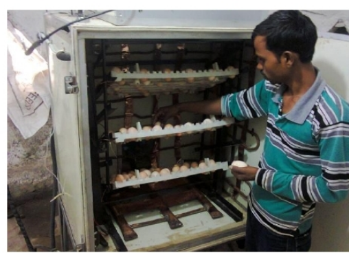
Solar Egg incubator live trial with 100 eggs
