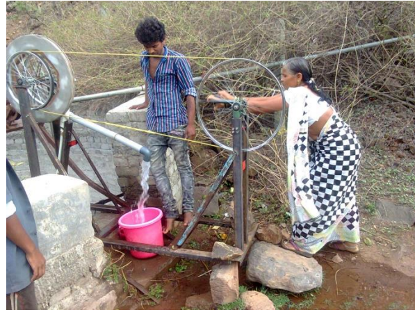
Testing washer pump on VA open well
