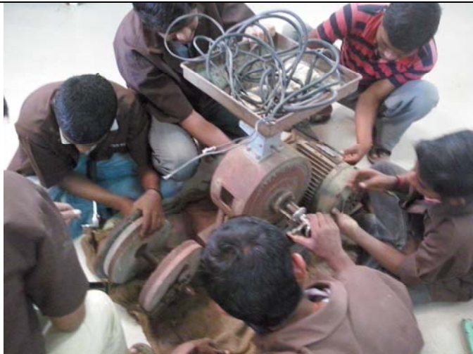
DBRT students repairing floor mill
